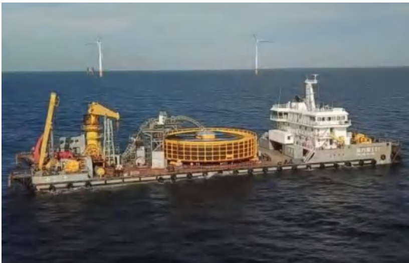
3500t Cable Laying Barge
